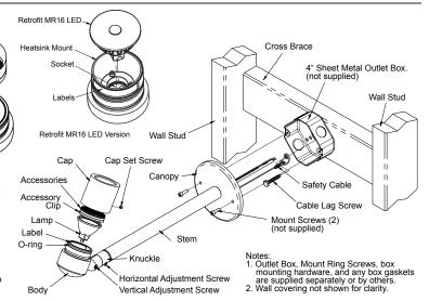
Do not use 'universal mounting rings' when installing this fixture. These rings are not capable of handling the weight and will most likely bend, causing 'sag' or potential failure. The canopy must mount directly to the box.
